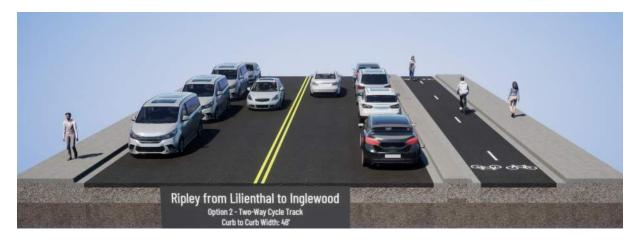
Figure 27 Proposed Section of Recommended Facilities for Ripley Avenue from Lilienthal Lane to Inglewood
