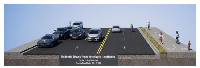
Figure 29 Proposed Section of Recommended Facilities for Redondo Beach Boulevard from Artesia Boulevard to Hawthorne Boulevard
