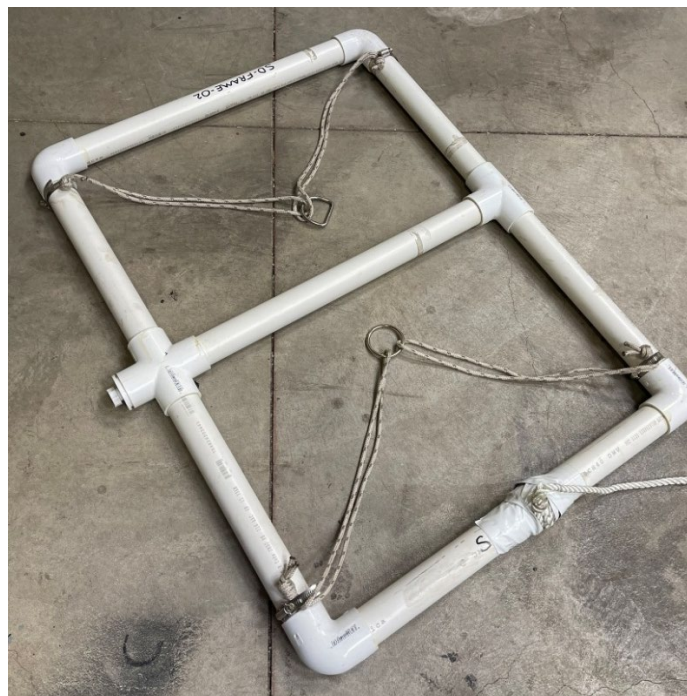
Figure 10. PVC Frame Used to Mount the RBR Wave Gauges.
