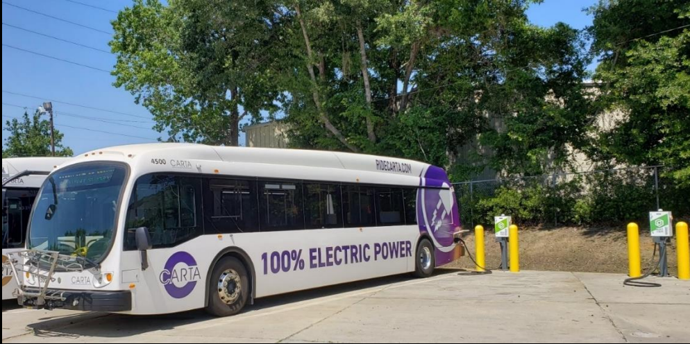
Example a BEB plugged into a charger
