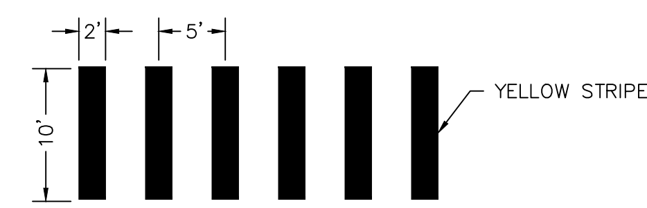
DETAIL B YELLOW CONTINENTAL CROSSWALK STRIPING NTS
