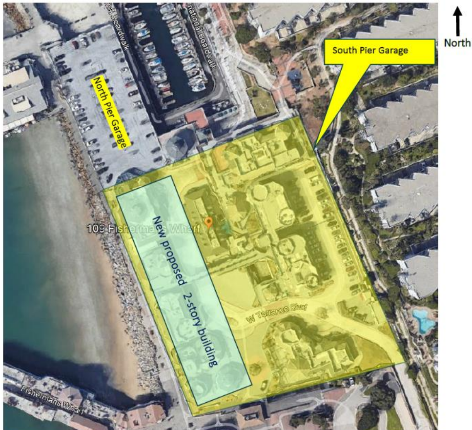
Figure. Approximate location of the new proposed structure on the top deck of the Redondo Beach South Pier Garage replacing the existing retail stores (20 ft distance from the west edge of the top deck extending along most of the length of the garage in the north-south direction).
