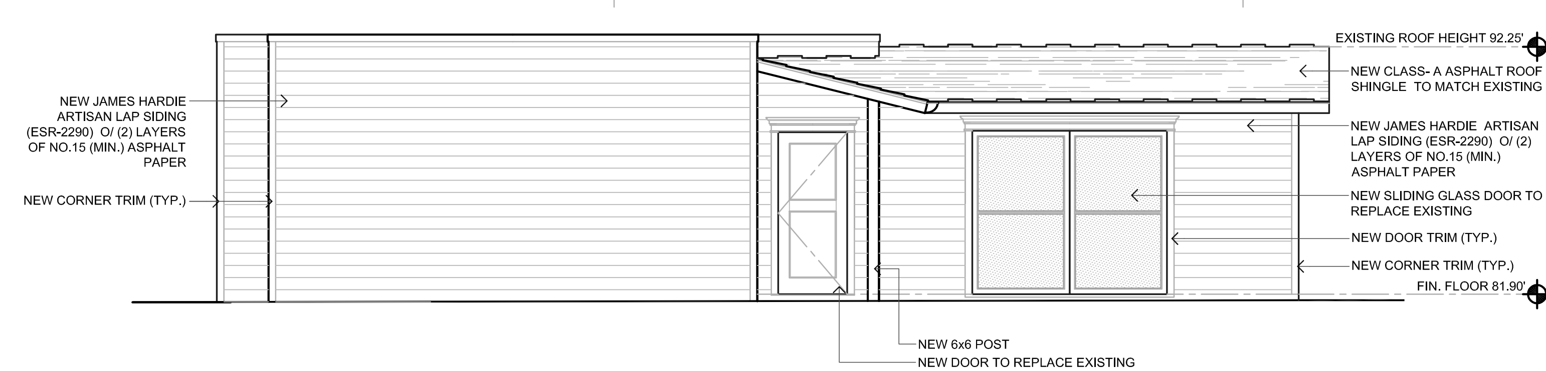
SOUTH GARAGE / ADU ELEVATION
