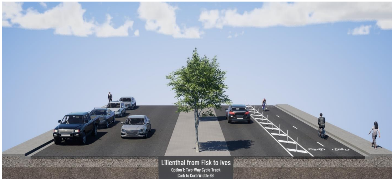
Figure 25 Proposed Section of Recommended Facilities for Lilienthal Lane from Lilienthal Park/Fisk Lane to Ives Lane
