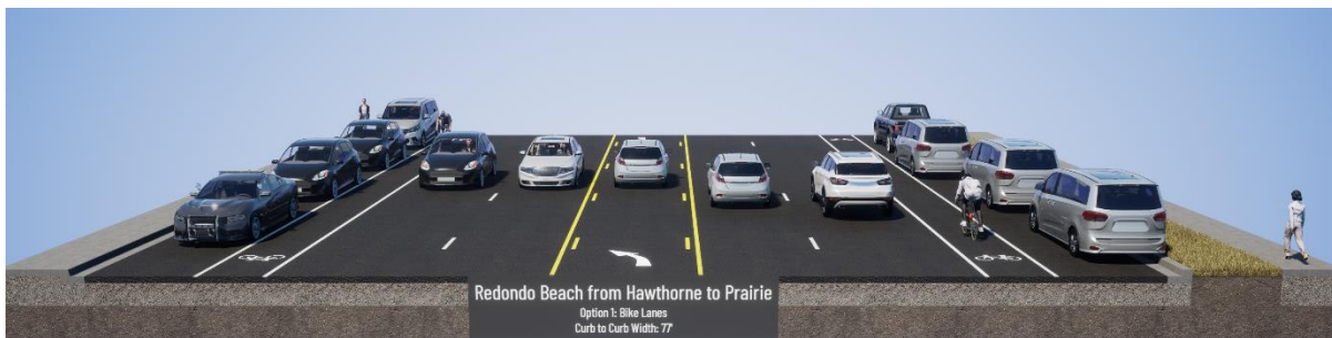
Figure 30 Proposed Section of Recommended Facilities for Redondo Beach Boulevard, from Hawthorne Boulevard to Ainsworth Avenue
