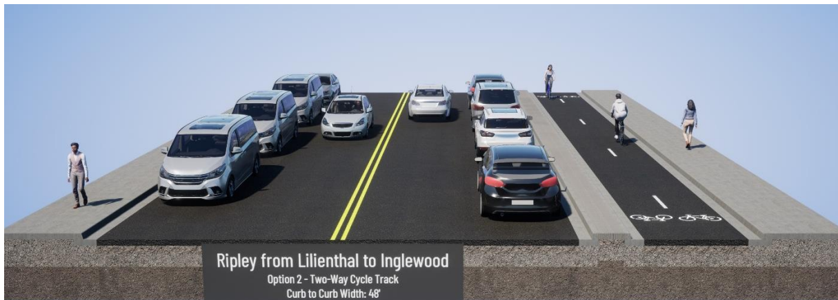
Figure 27 Proposed Section of Recommended Facilities for Ripley Avenue from Lilienthal Lane to Inglewood Avenue
