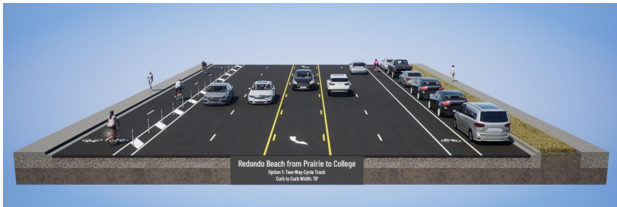
Figure 31 Proposed Section of Recommended Facilities for Redondo Beach Boulevard, from Ainsworth Avenue to Dominguez Channel
