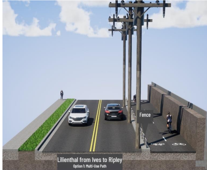
Figure 26 Proposed Section of Recommended Facilities for Lilienthal Lane from Ives Lane to Ripley Avenue
