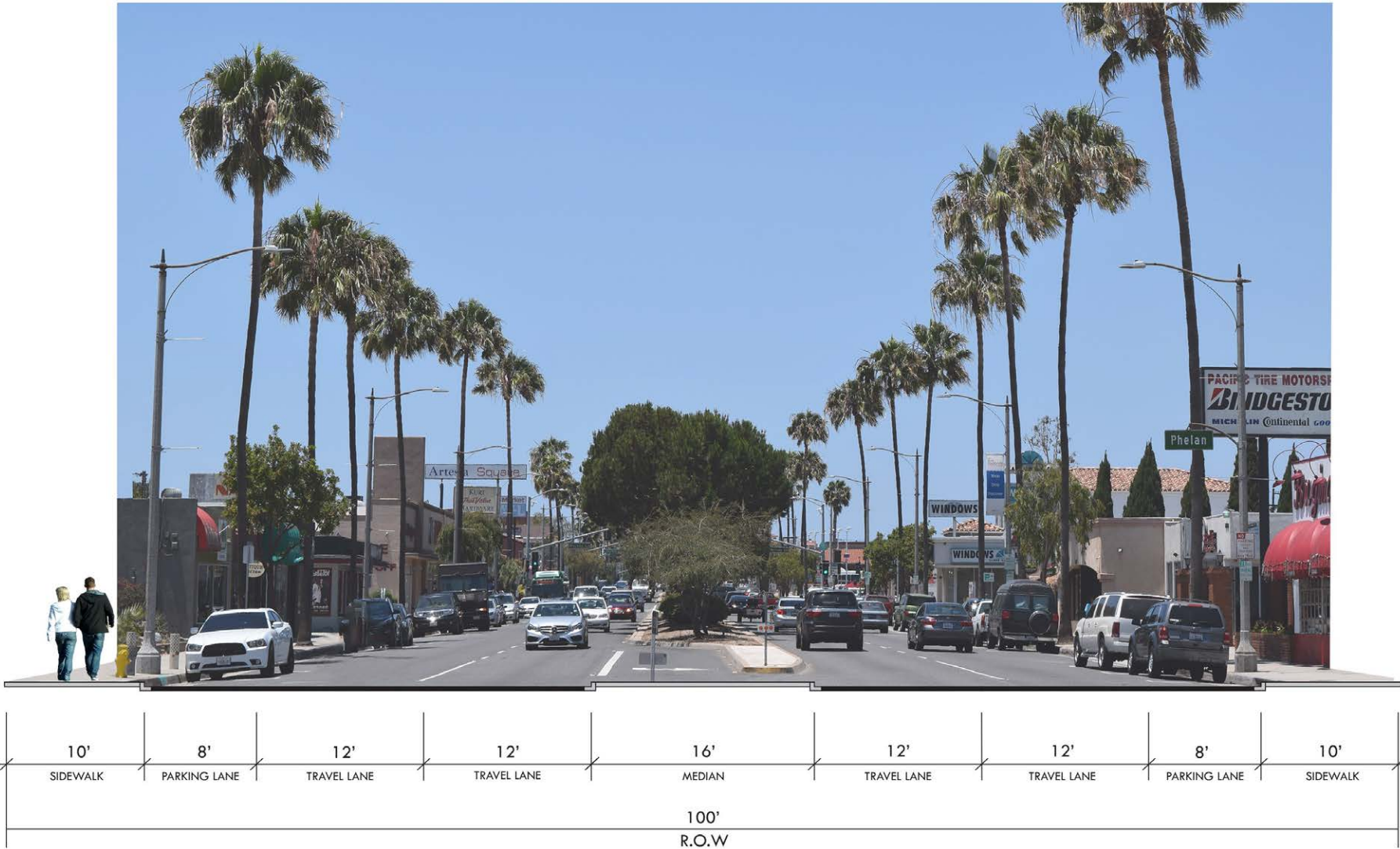
Figure 4.4: Artesia Boulevard Existing Configuration
