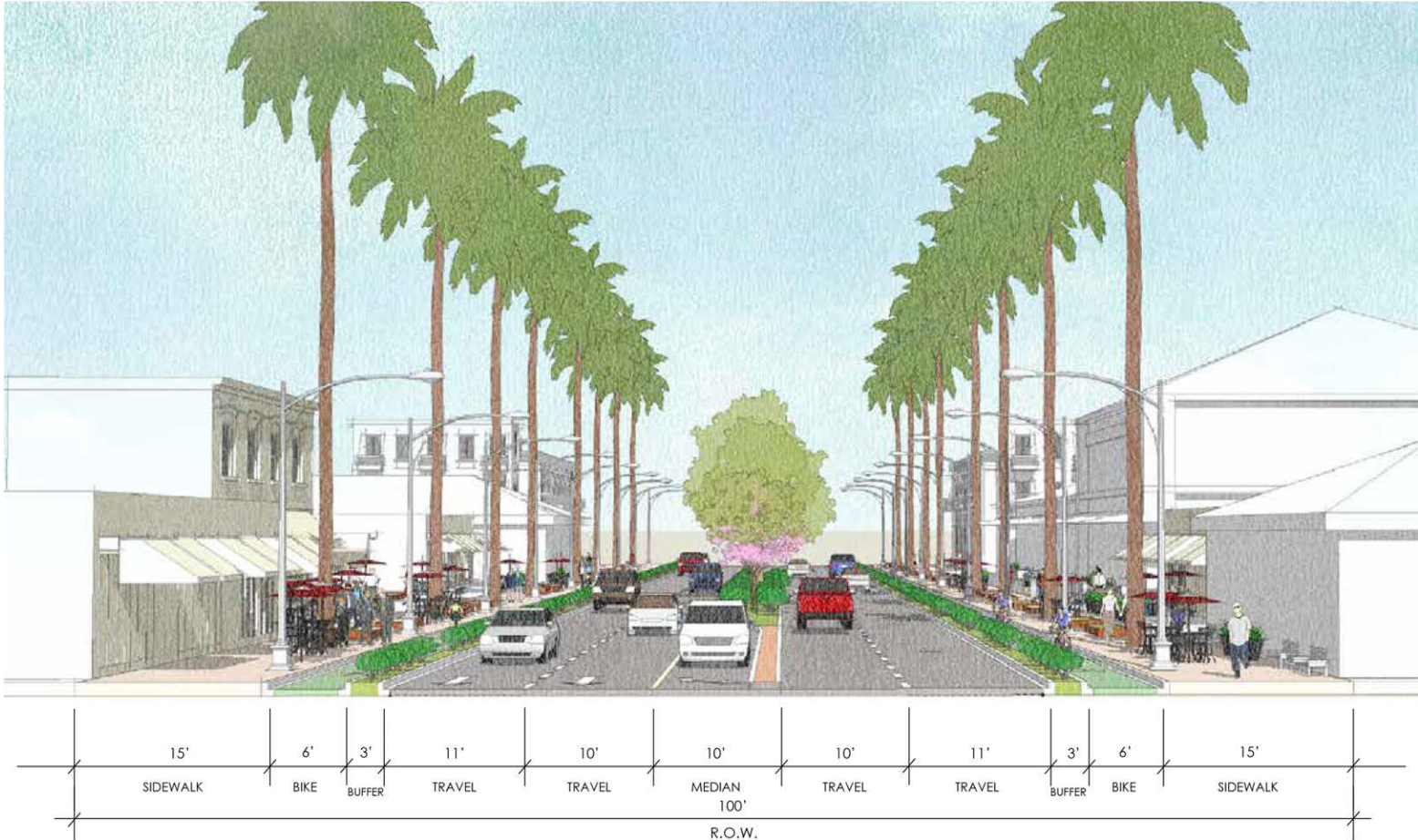
Figure 4.6: Artesia Boulevard Concept without Parking Lane
