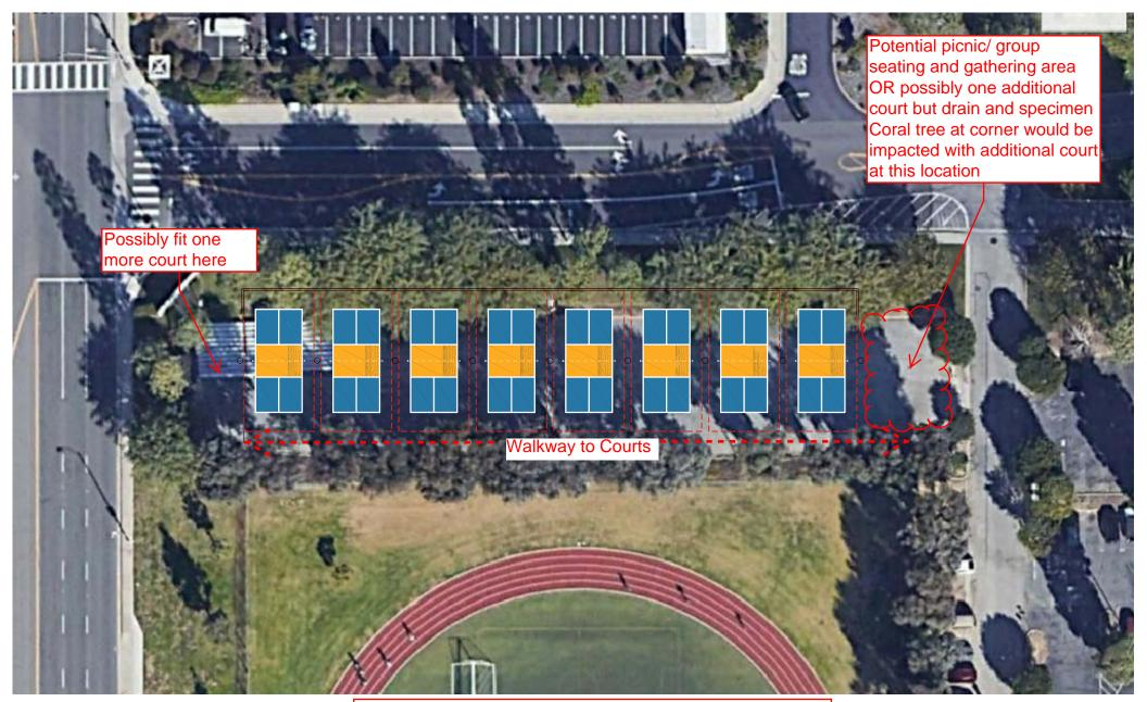
Possibilities of additional courts, up to 10 total, depending on drainage conditions and ease (cost) of modifying the existing drainage and utilities. 3-phase sports lighting may involve upgrading the electrical panel
