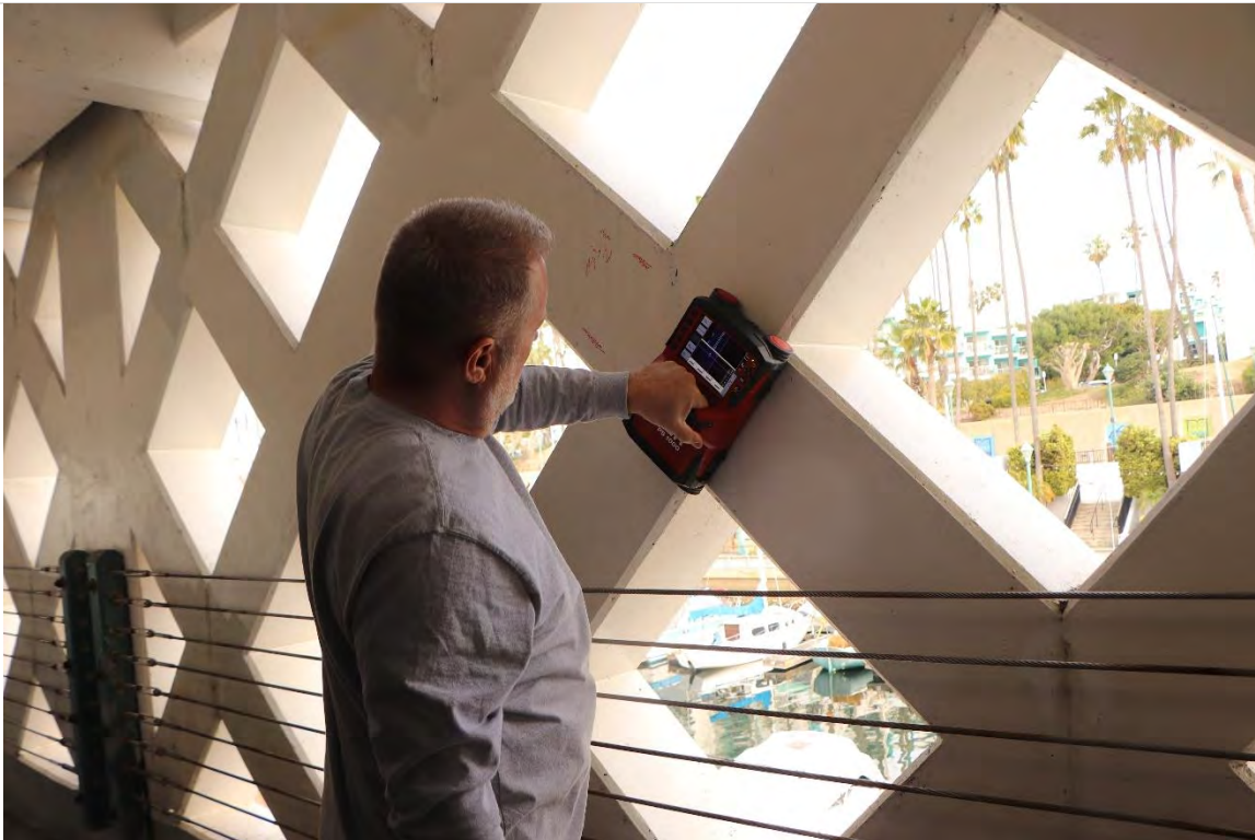
Photo 2.2- Detecting waffle wall steel reinforcement using GPR, East Wall, 1992 Retrofit – Pier Level (BA2-12)
