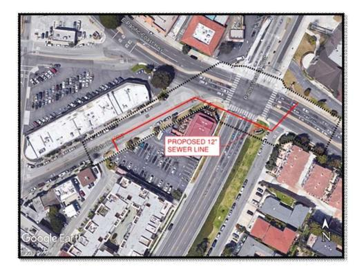
These improvements are designed to convey the increased sewer flow from future developments upstream of this connection within this sewer-shed, including the Legado Development.
