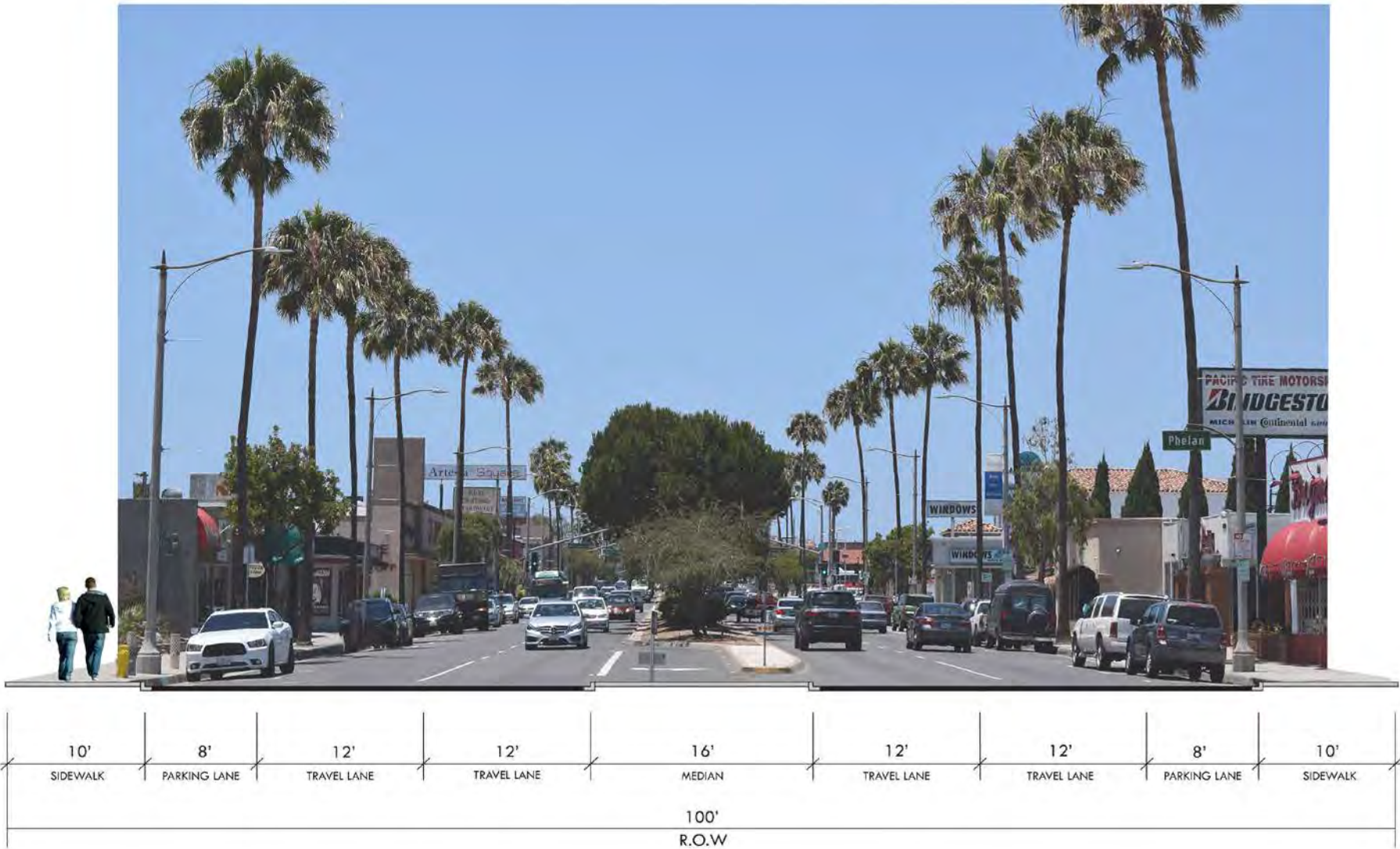
Figure 4.4: Artesia Boulevard Existing Configuration
