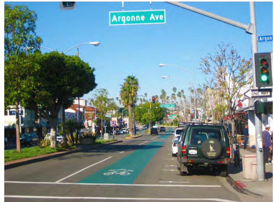
Example of a sharrow, which allows cars and bikes to share a vehicle lane.
