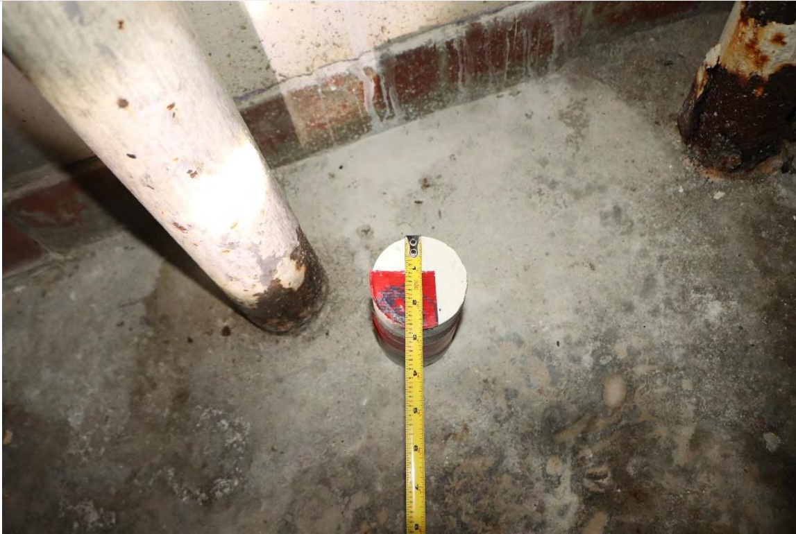
Photo 2.9- Typical concrete core, 3" diameter by 6" length, kitchen wall on gridline 3, 1962 Construction - Basement (BA2-224 and 226)
