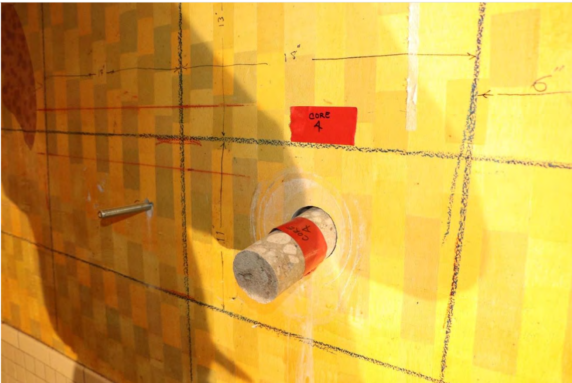
Photo 2.8- Concrete coring, Kitchen wall at gridline 3, 1962 Construction - Basement (BA2-96)
