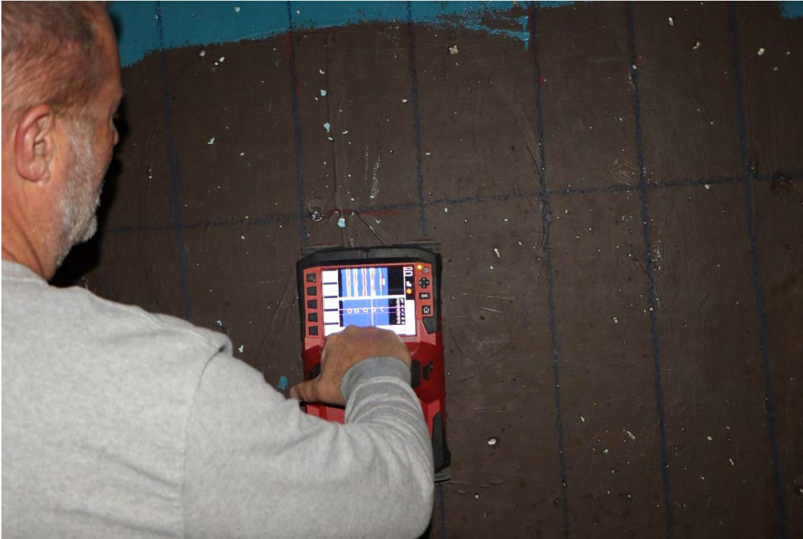
Photo 2.1- Detecting wall steel reinforcement using GPR, West Wall, 1962 Construction - Basement (BA2-9)
